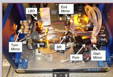
Figure 4: Early Laboratory Demonstrator of a 589nm OPSL (Credit: Areté Associates)
