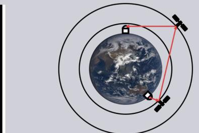
Figure 8: Principle of Ground-Satellite, Satellite-Satellite, and Satellite-Ground Laser Communications
