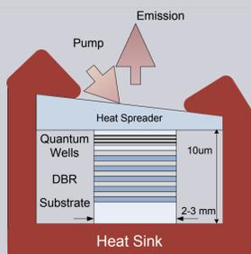
Figure 3: Semiconductor Laser Gain Medium (Credit: Areté Associates)
