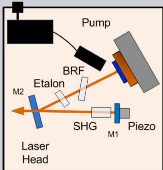
Figure 1: Semiconductor Guidestar Laser Cavity Layout (Credit: Areté Associates)
