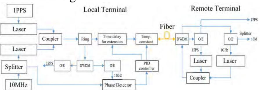
Fig.2 The principle of fiber-optic time-frequency transfer
