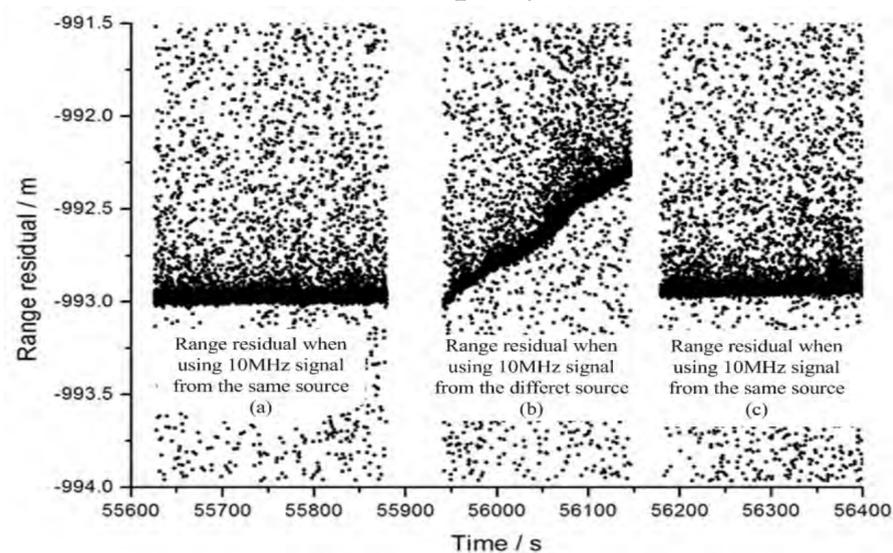
Fig.4 The range residual of Glonass128 from 1.56m telescope Comparing the observation range after calibration with the precise orbit of satellites, the range bias of data from the 1.56m telescope was less than 6cm in figure 5, allowing for satellite orbit determination.
