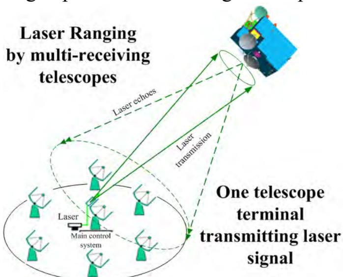
Fig.1 The one telescope terminal transmitting and multiple telescopes receiving laser signal
