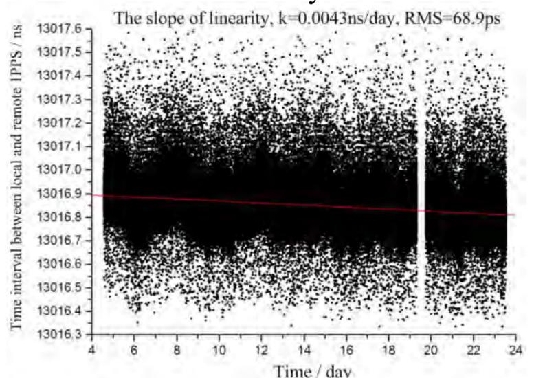
Fig.3 The stability of fiber transfer link between local terminal and remote terminal
