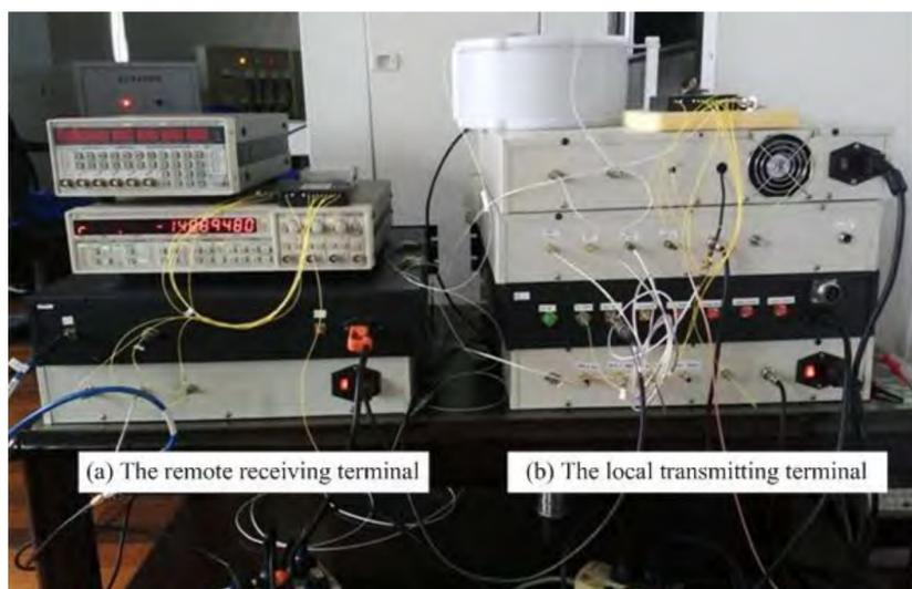
Fig.3 The device of fiber-optic time-frequency transfer
