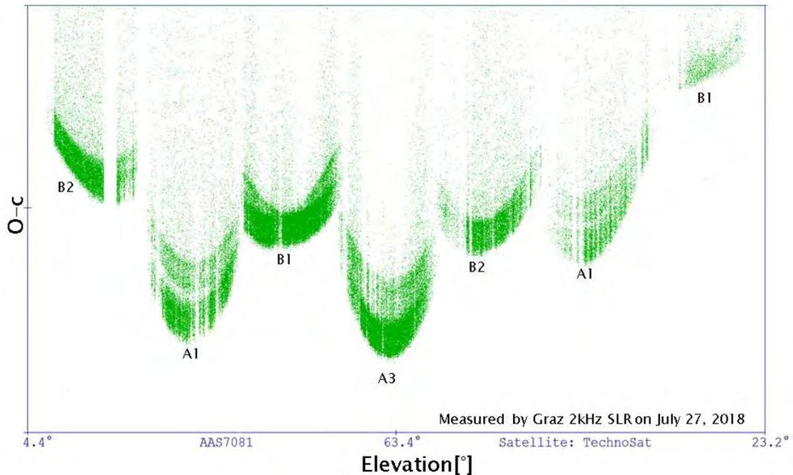
**Figure 8:** TechnoSat spin in the sequential order of B2 → A1 → B1 → A3 → B2 → A1 → B1
