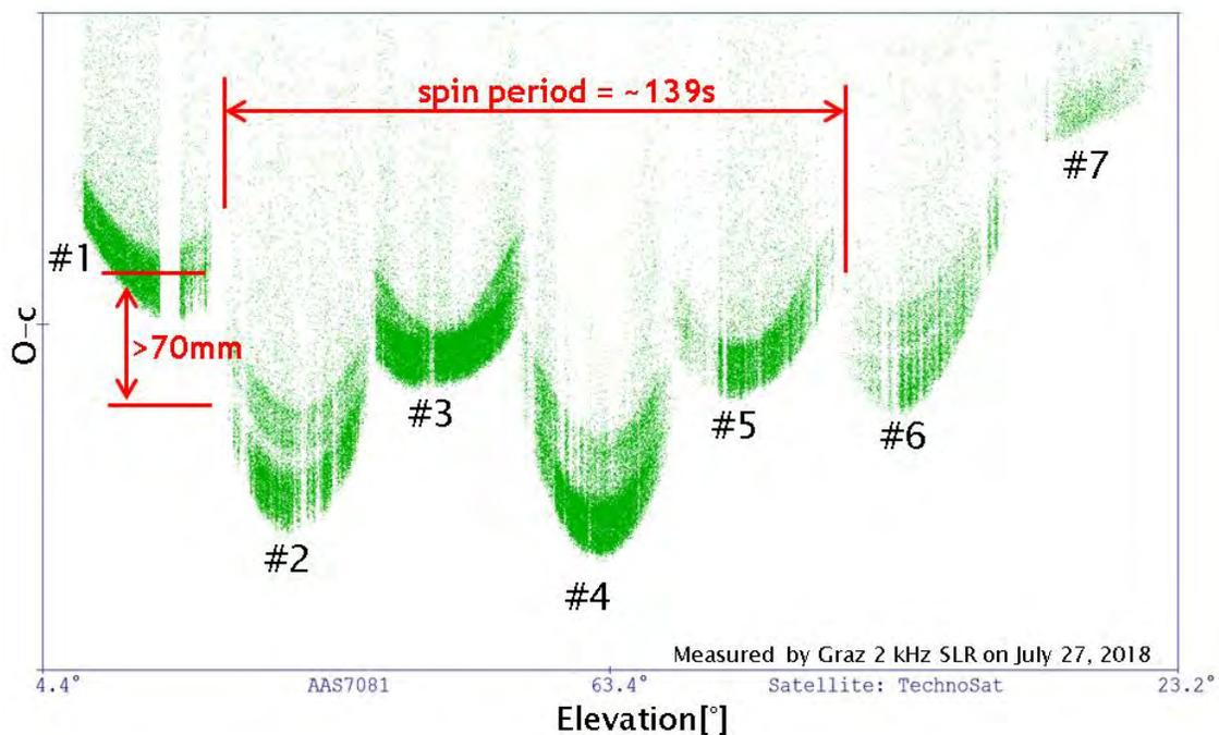
**Figure 5:** Seven faces of TechnoSat tracked by the 2 kHz laser ranging system in Graz while spinning with a period of approximately 139s
