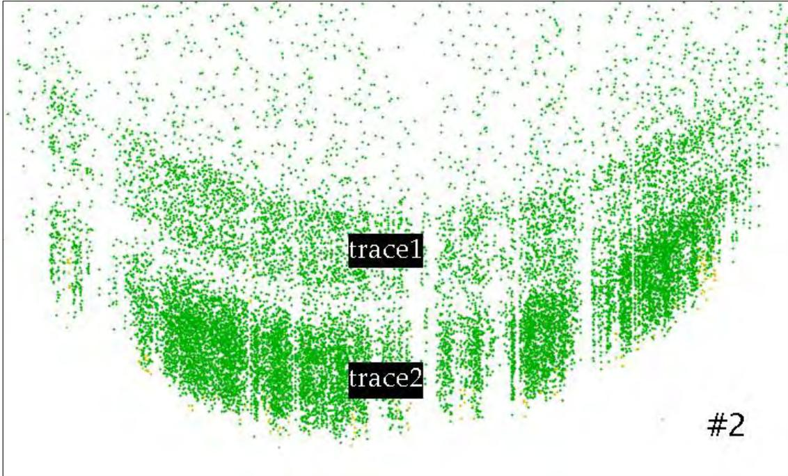
**Figure 6:** Two traces of laser returns, where the RMS and signal density of trace1 are less than of trace2
