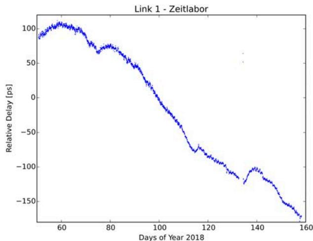
*Fig. 4: Error signal of the long-term stability of the compensated time and frequency fiber link. Over a period of more than 100 days a delay variation of more than 350 ps has been taken out by the closed loop system.*
