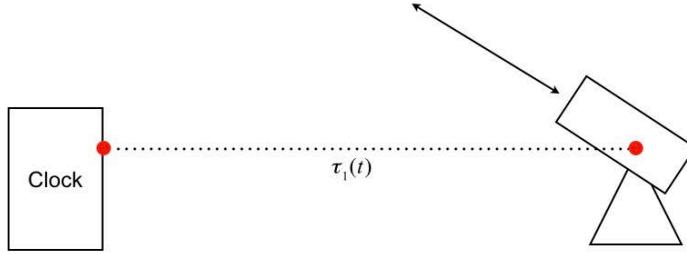
*Fig. 2: Accurate time transfer requires the exact knowledge of the time delay between the point of reference at the clock and the effective reference point of the SLR system, performing the time transfer. In most cases this offset will vary in time, due to the electronic systems and cable runs involved in the transport of the timing signals.*
