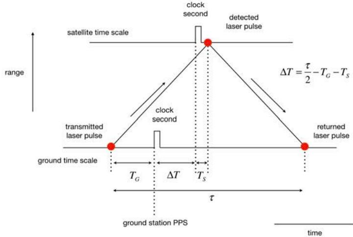
Fig. 1: Illustration of the optical time transfer process, between a timescale on the ground and in space. The horizontal axis indicates time, while the ordinate represents the distance between the timescales.
