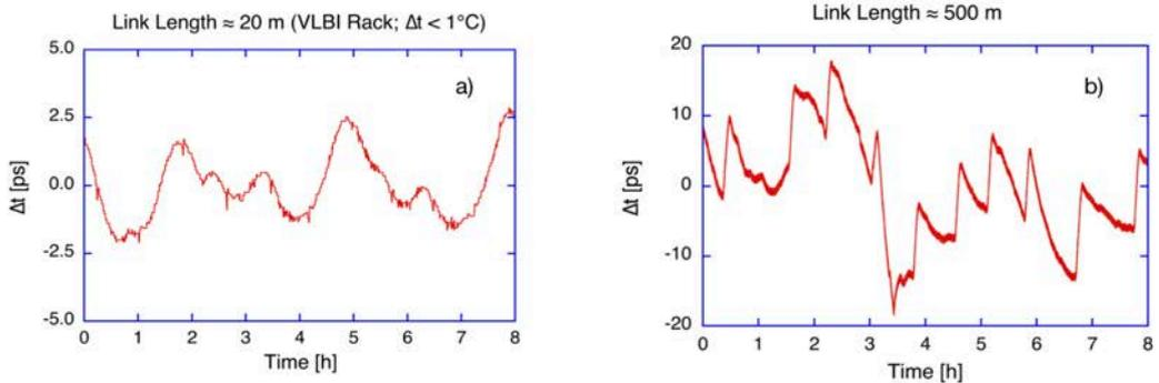
*Fig. 3: Short-term stability of the local time and frequency distribution. The compensated delay variation is taken from the error signal of the closed loop delay compensation. A variation of only several picoseconds is observed for a short lead of 20 m, running inside an air conditioned room a). Considerably larger delays are found for a 500 m long run of fiber, connecting 2 different buildings b).*
