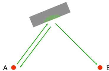
Fig. 1 laser time transfer between two stations by diffuse reflections from a rocket body. Each station performs two-way ranging to the rocket body. In addition to that, each station performs one-way detection of the laser pulses from the respective other stations. That is: 1 shot fired per station and 2 returns detected.
