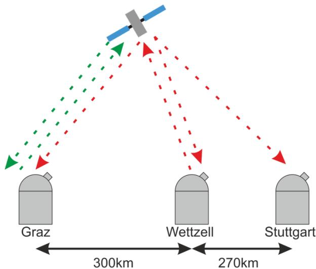
Figure 1 Realized measurement configurations. Red arrows indicate ranging at a wavelength of 1064nm, whereas green arrows indicate ranging at a wavelength of 532nm.
