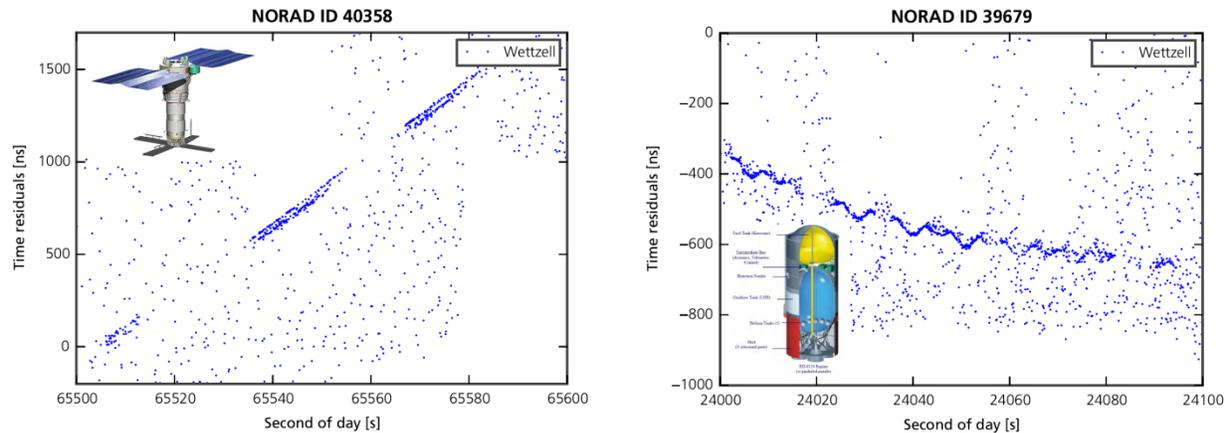
Figure 3 Left: Residual plot of object 40358. Two distinct lines are visible, which are separated by about 35ns. Inset from [4] Right: Residual plot of object 39679. An oscillation is visible with an amplitude of 30ns and a period of 11.5s. Inset from [5].
