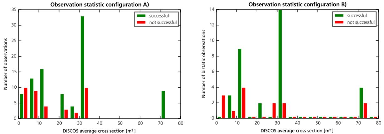
*Figure 2 Successful/not successful ranging attempts as function of the average object cross section for configuration A and B. The target cross sections are extracted from ESAs DISCOS catalog.*
