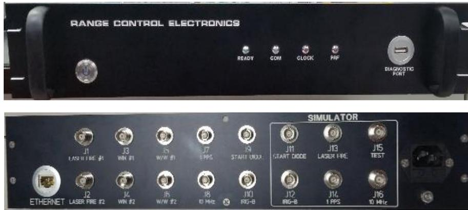
Figure 5 - Front and Back View of RCE Chassis
