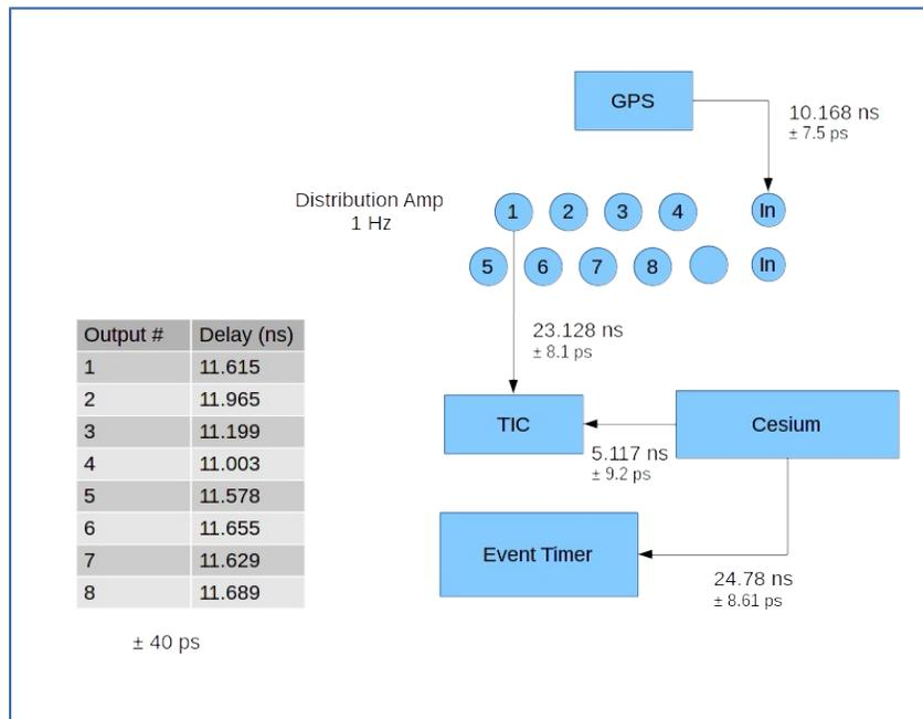
Figure 4: Tracing Cesium 1 PPS to UTC
