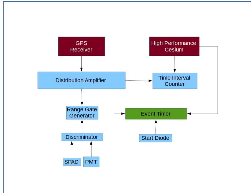
Figure 1: Simplified Timing Block Diagram
