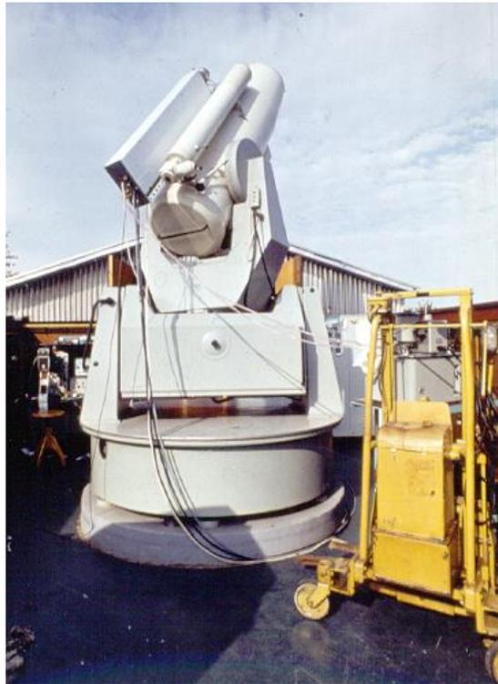
Fig 1: SBG camera with laser head and collimator installed, laser power and cooling electronic on the right side
