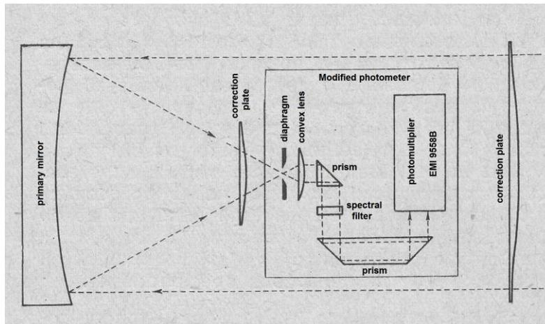
Fig 2: Scheme of detection package – modified photometer – installed in focal plane of SBG camera (from [3])
