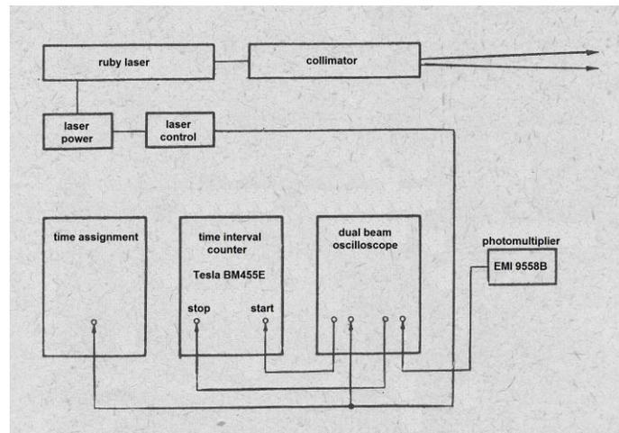
Fig 3: Signal scheme of experiment (from [3])
