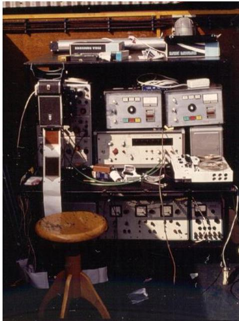
Fig 4: Detection electronic. In the middle from left to right: dual-beam oscilloscope with photographic recording, time interval counter, magnetic tape recorder for voice recording
