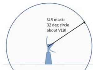
**Figure 4:** SLR pointing exclusion mask to prevent damage to VLBI from SLR radar.
