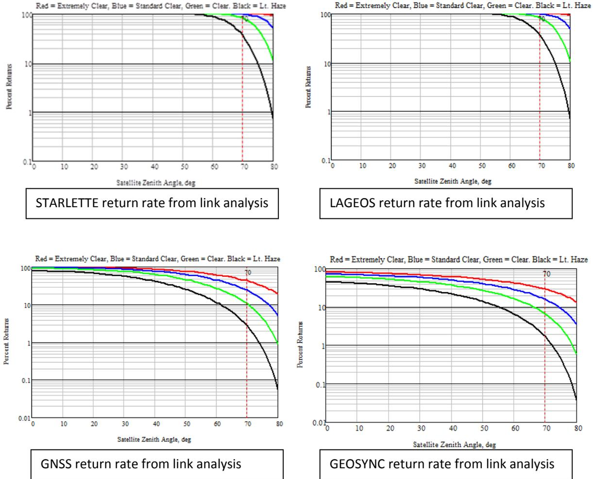
**Figure 3:** Link analysis based upon SGSLR design shows high return rates for all satellites. System characteristics used: laser divergence = 7 arcseconds for LAGEOS, GNSS and GEO, and 12 arcseconds for STARLETTE; per pulse transmit energy = 1.5 mJ; telescope aperture = 0.5 m. No pointing error. Curve colors represent atmospheric clarity: RED is extremely clear; BLUE is standard clear; GREEN is clear; BLACK is light haze.
