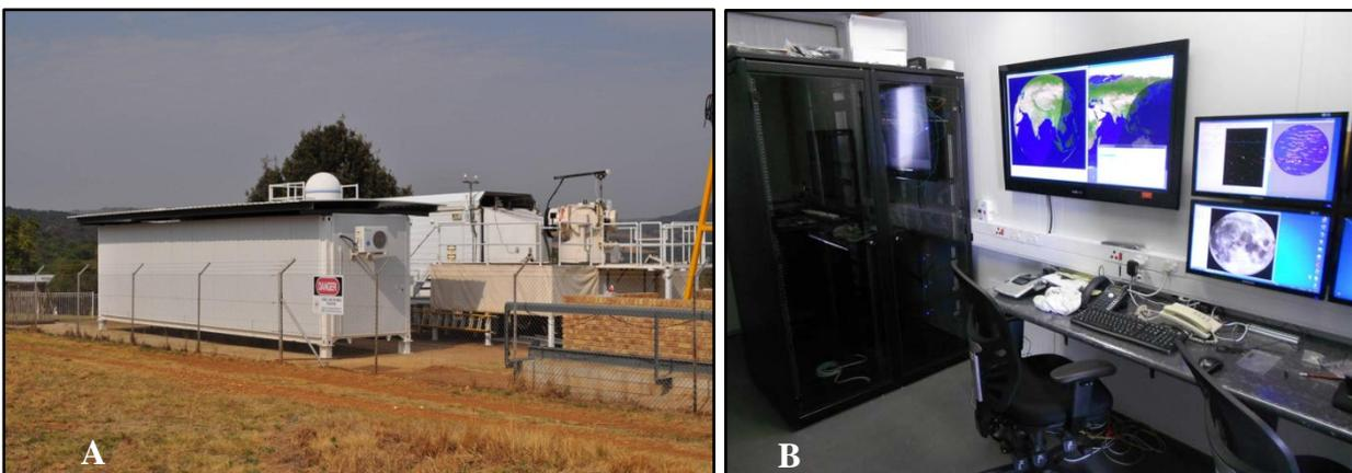
**Figure 5.** (A) The modified shipping container which is utilized for the control centre. It has been fitted with a shade providing roof. (B) Two standard 19" racks will contain all the electronics and the operator will track the Moon and satellites using only a mouse and keyboard.
