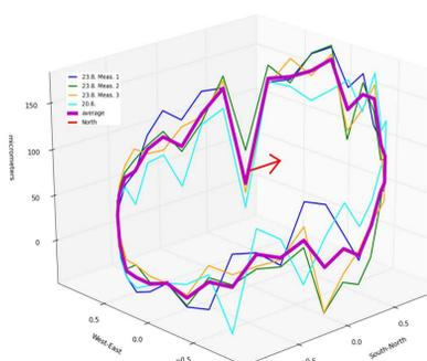
Figure 4. Plot showing levelled height differences. The starting point is set to zero. Magenta is the total average, other colors are the averaged separate measurements.
