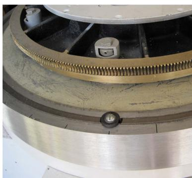
Figure 3. The azimuth rail. Black marks show the levelled points. The rod was placed on the magnet to reduce error due to placing of the rod on the rail.
