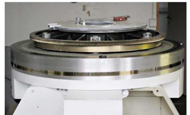
Figure 2. The gold plated scale of the azimuth encoder mounted on the telescope mount.
