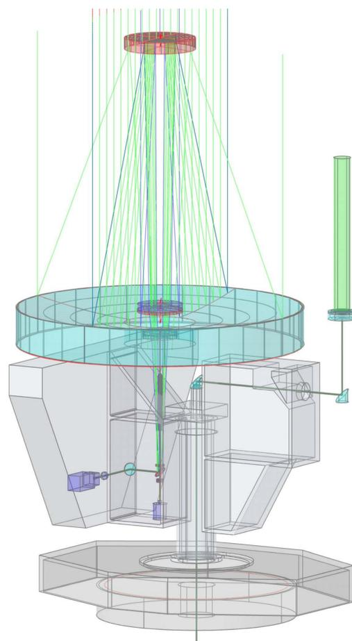
Figure 1. CAD-drawing of the telescope mount and the new optical setup. The green color shows the laser beam; magenta illustrates the detectors and red and turquoise shows the optics. The three new custom lenses are mounted to the hole in the middle of the main mirror.
