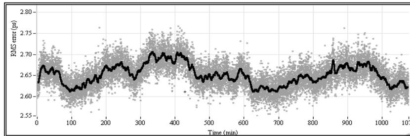
**Figure 2. RMS resolution vs. time under ambient temperature variation in the range  $\pm 2.5\text{ }^{\circ}\text{C}$**
