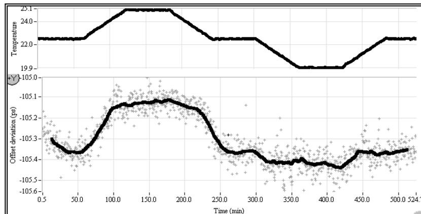
Figure 5. Input-to-input offset drift in line with slow linear changing of ambient temperature from 20 to 25  $^\circ\text{C}$
