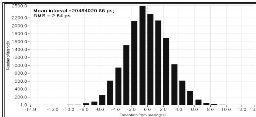
Figure 1. Histogram of time intervals measured by the A033-ET
