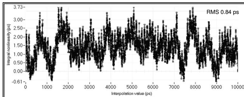
**Figure 3. Integral non-linearity error over 10 ns interpolation interval**
