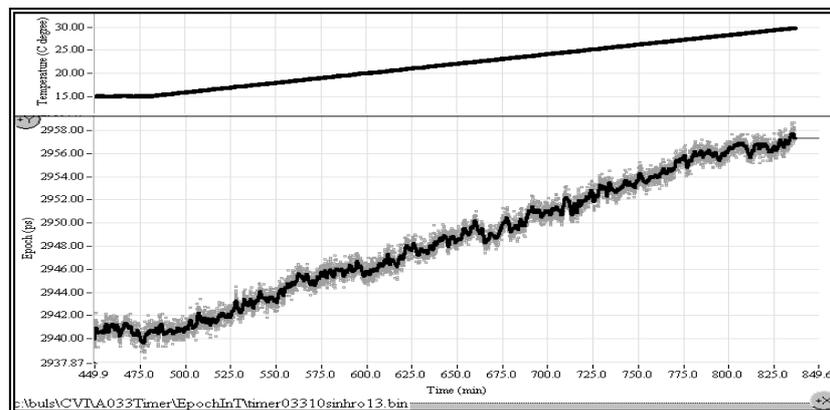
Figure 4. Single-input offset drift in line with slow linear changing of ambient temperature from 15 to 30  $^\circ\text{C}$
