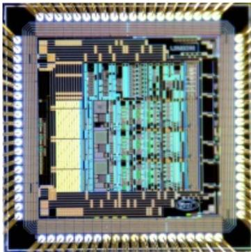
Fig. 1. Bare chip of prototype IC (LIDARX03)
