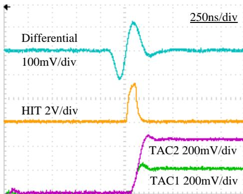
Fig. 3. Typical output waveforms from LIDARX03
