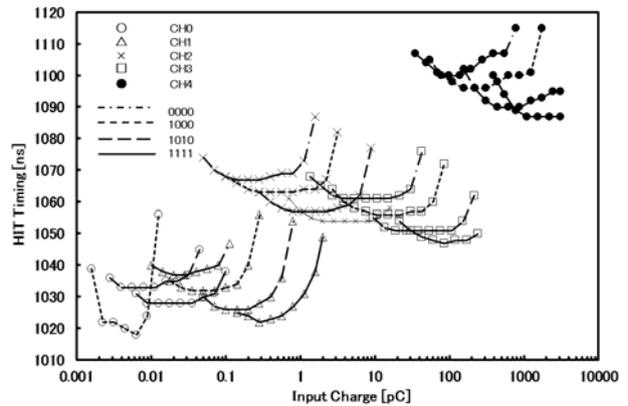
(a) Detected pulse timing
