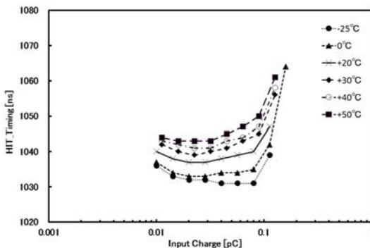
Fig. 5. Temperature dependence of detection timing
