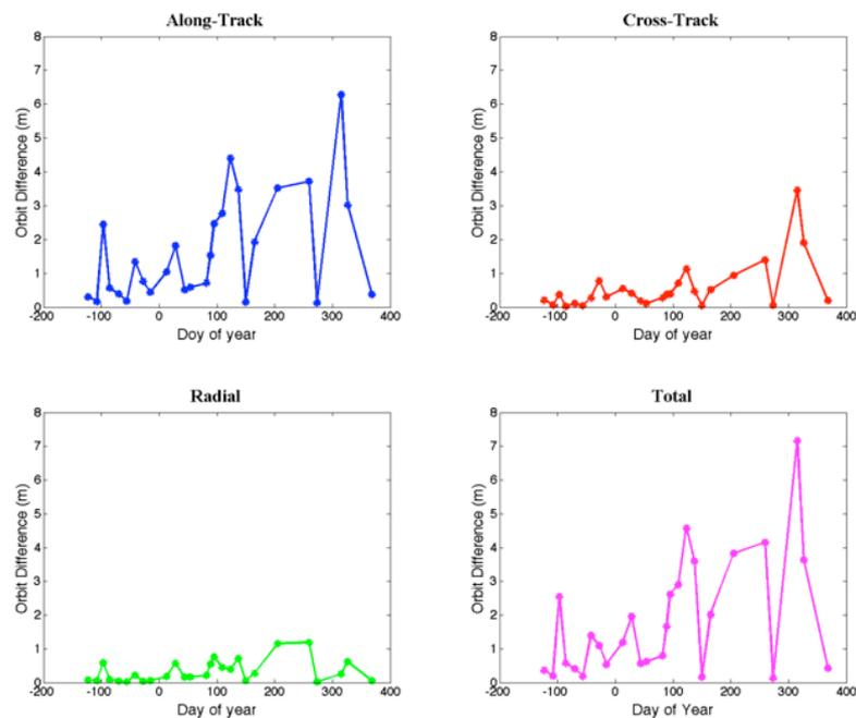
**Figure 5 Orbit difference between GEODYN calculations with and without LR data in three directions, along track (blue), cross track (red), radial (green), as well as the total orbit difference (magenta).**
