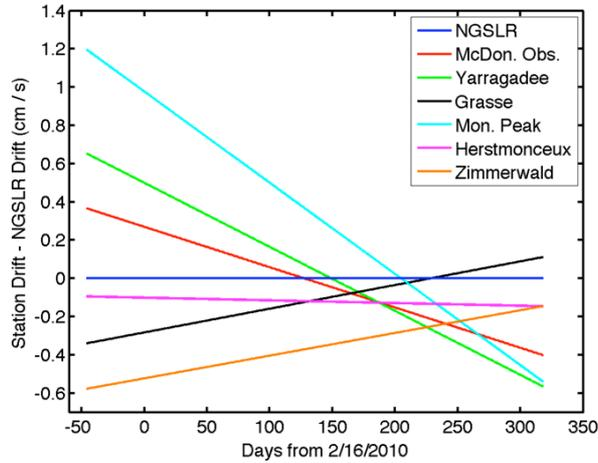
Figure 3 LRO clock drift rate for different LR stations relative to NGS LR.
