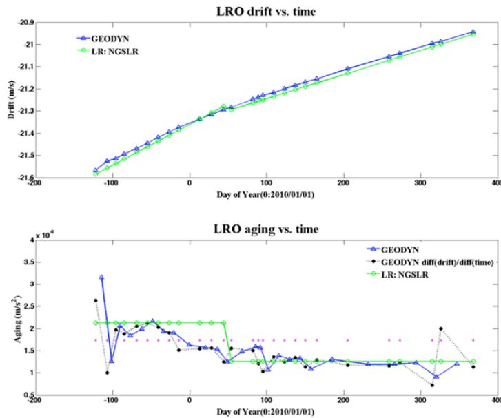
Figure 2 Long-term LRO clock stability derived from LR data (green) and GEODYN estimation (blue), and the aging rate from pre-launch testing (magenta) plotted as a constant.
