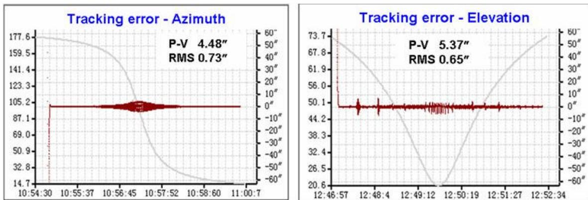
Figure 3 Tracking error of 1 meter aperture telescope, RMS<1 arc second
