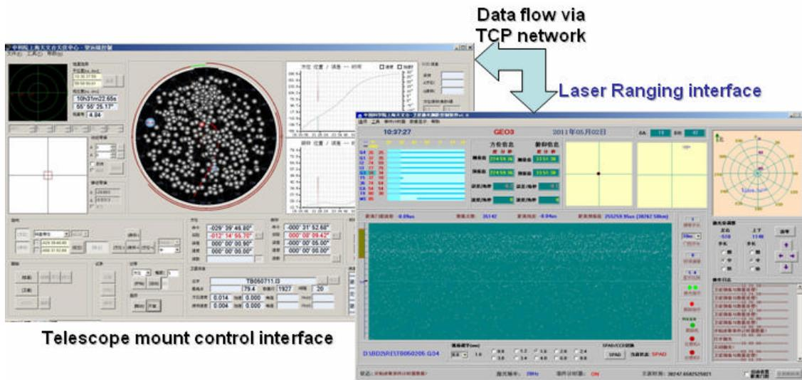
Figure 2 The software interface of laser ranging and telescope mount controlling
