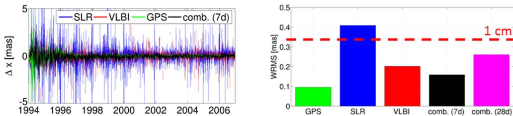
**Fig. 4:** Left: X-component differences of the terrestrial pole w.r.t. the IERS 08 C04 time series. There are displayed the technique-only solutions SLR, GPS and VLBI and the combined solution with a seven day arc length; Right: WRMS values of the differences of the technique-only solutions and both combined solutions (7-day/28-day).
