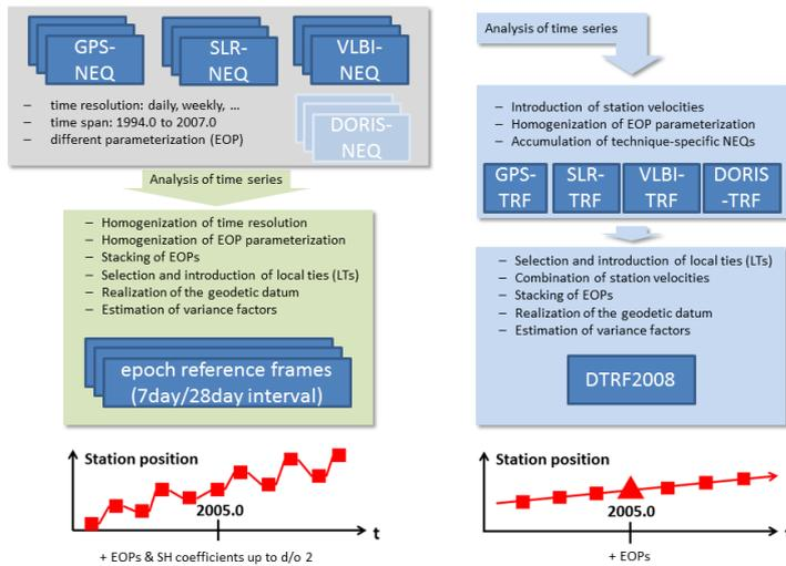
Fig. 2: Processing scheme for epoch and multi-year reference frames.
