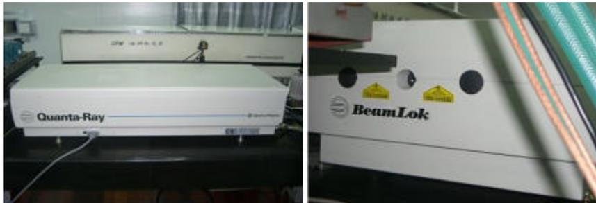
Figure 5 The view of 10W power laser
