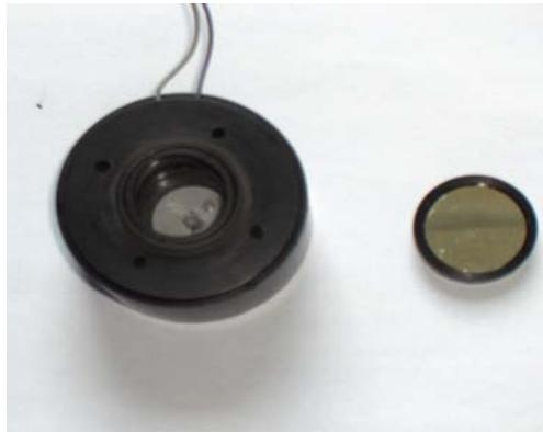
Fig.2 Spectrum filter in constant temperature box
