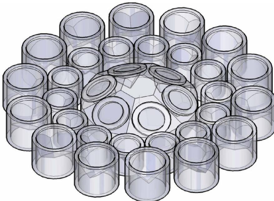
**Figure 4.** Basic design of ASTRO-G retroreflector array.
