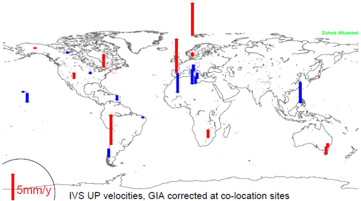
**Figure 7.** Vertical velocities of IVS-VLBI (intrinsic scale and ITRF2000 origin) co-located stations, corrected by ICE-5G V1.2 GIA model of Peltier (2004). Red vectors represent positive velocities and blue vectors negative velocities.
