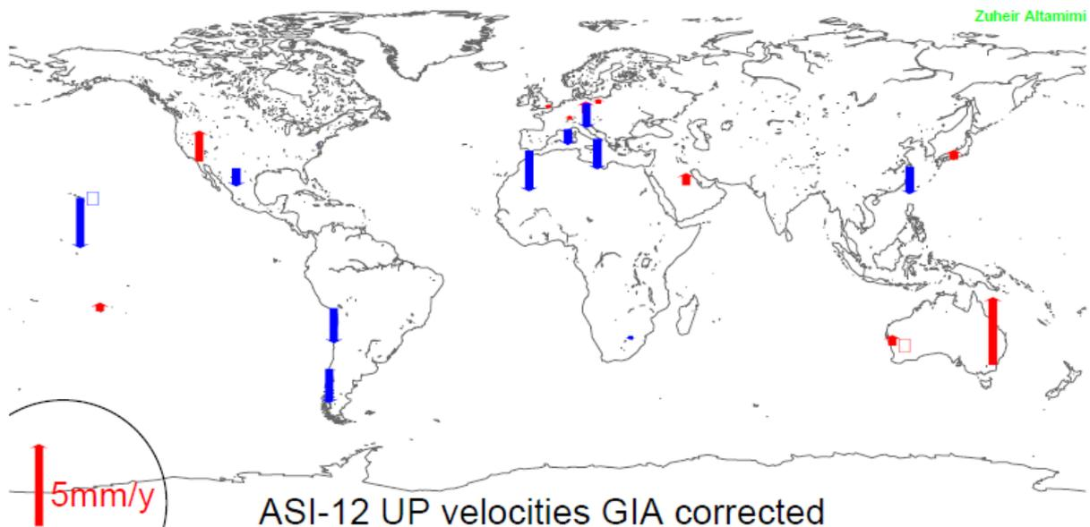
**Figure 5.** Vertical velocities of ASI-12 SLR core network, corrected by ICE-5G V1.2 GIA model of Peltier (2004). Red vectors represent positive velocities and blue vectors negative velocities.
