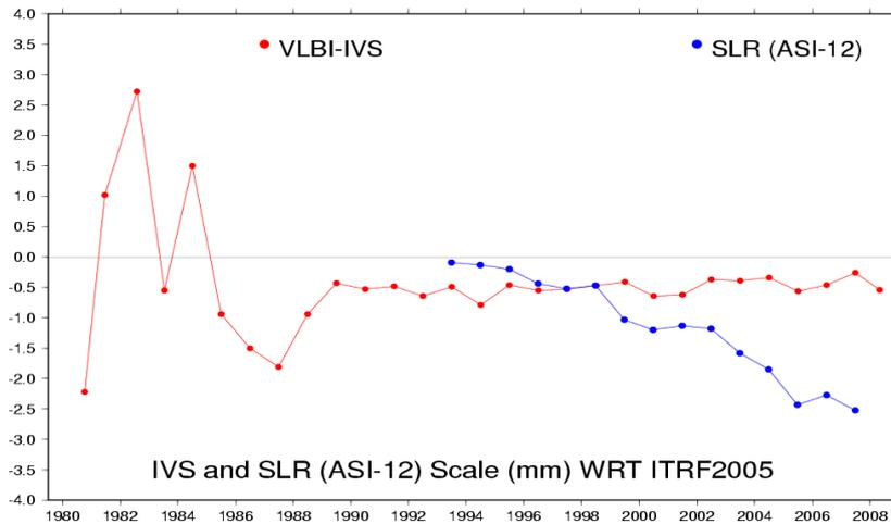
**Figure 3.** Averaged annual scale factors of VLBI IVS and SLR ASI-12 time series with respect to ITRF2005
