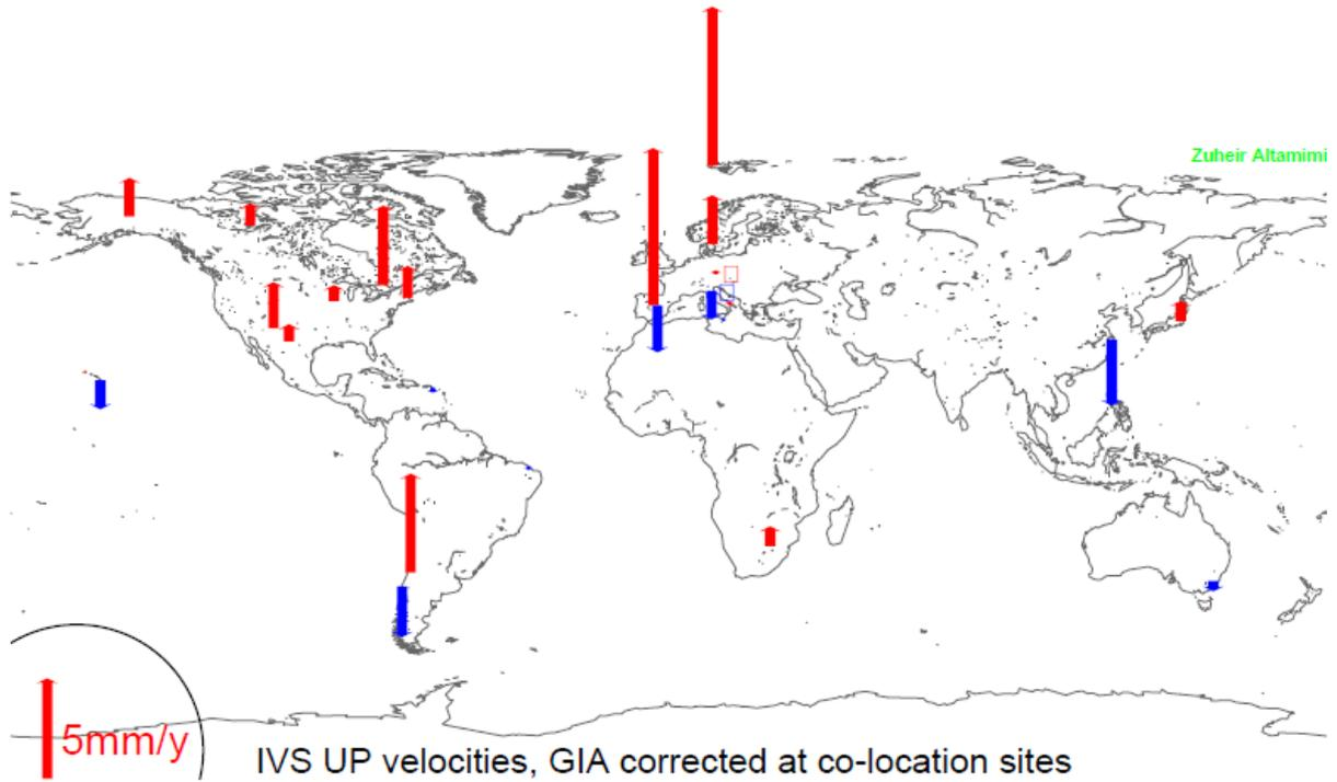
**Figure 6.** Vertical velocities of IVS-VLBI (intrinsic scale and ITRF2005 origin) co-located stations, corrected by ICE-5G V1.2 GIA model of Peltier (2004). Red vectors represent positive velocities and blue vectors negative velocities.
