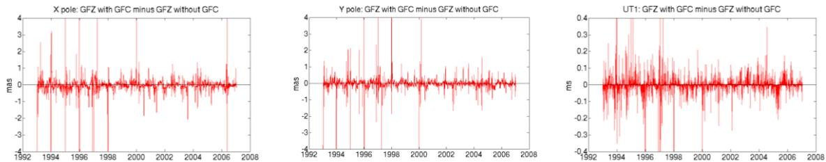
**Figure 10.** ERP differences between GFZ GGOS-D solutions with fixed gravity filed coefficients and estimated ones: x-pole (left), y-pole (middle), UT1 (right)
