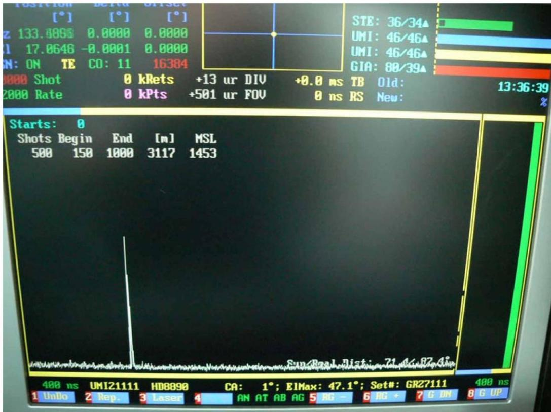
Figure 2. Real Time Display of Graz kHz LIDAR: A strong backscatter signal at 3117 m distance, from a cloud in 1453 m altitude (MSL); full daylight, single photon detection
