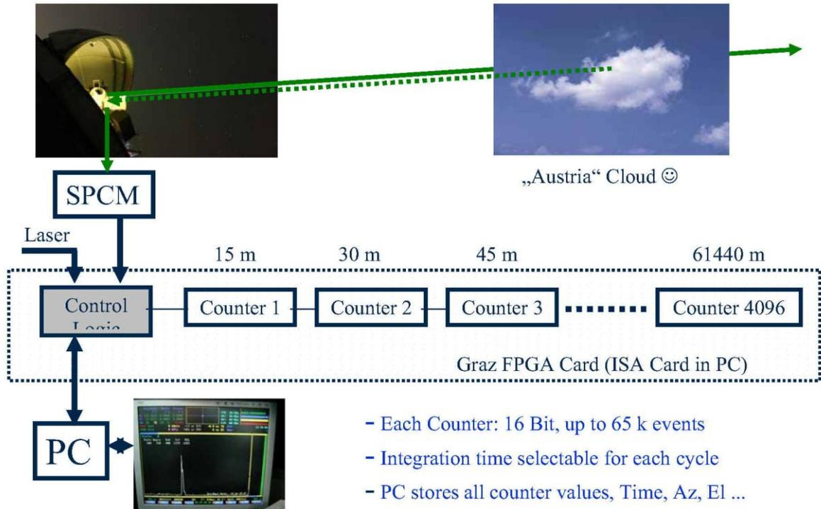
Figure 1. Schematics of Graz kHz LIDAR Hardware
