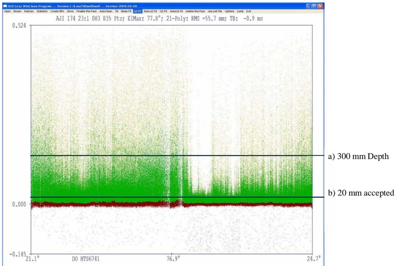
To use the inherent accuracy of our kHz system, but still keeping the operational simplicity and the high return rates, we are using now the "Leading Edge" (LE) of the returns as a reference line, and accept only returns from the first 20 mm reflective depth during post processing. Returns from behind this 20 mm limit are rejected. Although this method reduces the total amount of accepted returns (average reduction: about 30%), it offers significant improvements:
