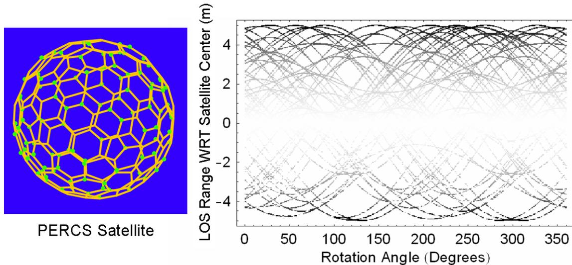
**Figure 3.** Coding of the PERCS retro-reflector locations to yield the orientation of the sphere in sphere. The line-of-sight (LOS) returns for a ground laser pulse provide unique time sequence depending on which side of the sphere is facing the viewer.
