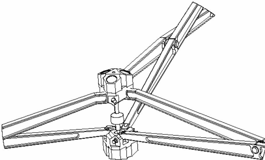
**Figure 2.** Retro-reflector holders for 1-cm corner-cubes on each PERCS vertex.
