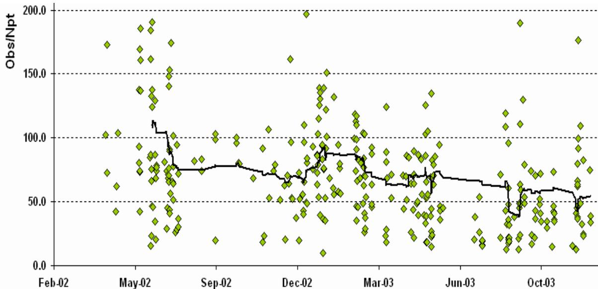
**Figure 1.** Number of observations per normal point at 423.5 nm during TIGO's first two years of operation. The return rate has fallen by approx. 50 % in less than two years, presumably due to the degradation of optical components.
