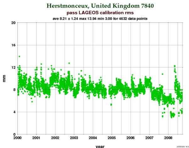
There is a clear drop in RMS at the beginning of 2007 on the installation of the event timer. A further drop in RMS is present for later passes, indicating kHz observations. The later higher RMS passes are due to the temporary use of an older SPAD detector.
