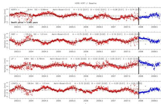
The new site between HERS and HERT, locally called SOLA, identified the poor data quality from the HERT Z-18 receiver. A new Lecia receiver was initially sited on the SOLA pillar and then later switched with the HERT Z-18 receiver bringing the observed signal noise to the SOLA site. Hopefully in time this additional site will also explain the annual variation in the baseline.
