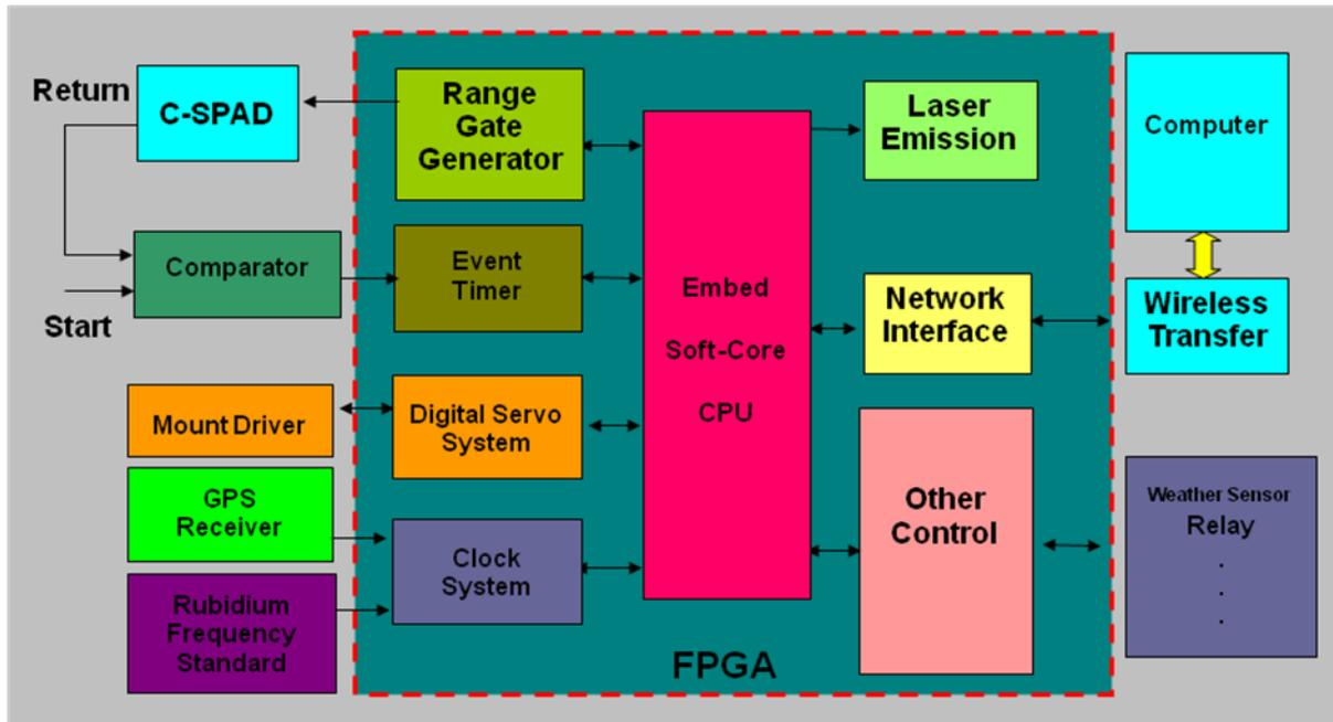
Figure 2. TROS FPGA board for KHz laser ranging
