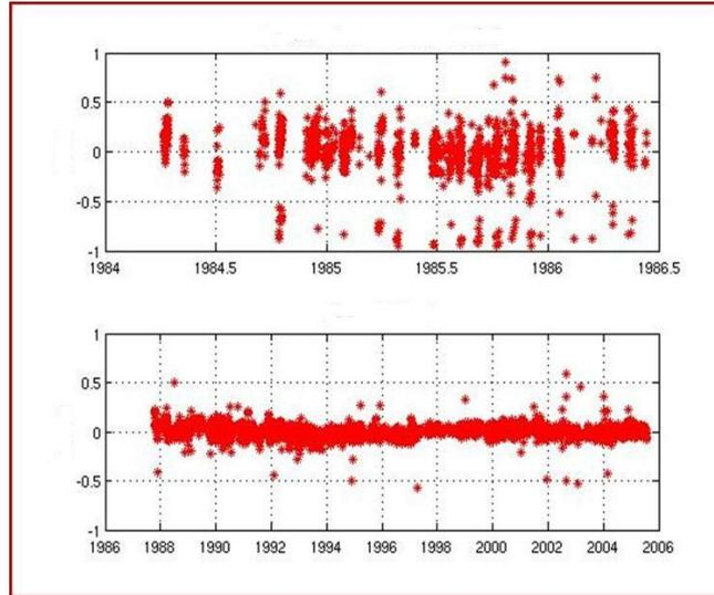
**Figure 1.** LLR residuals of Grasse station from 1984 to 2006 (in meters)
