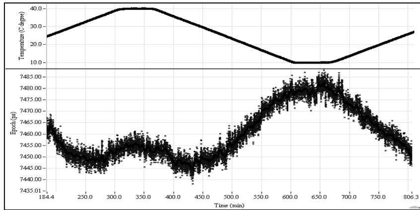
**Figure 5.** Internal time-base instability vs. ambient temperature variation
