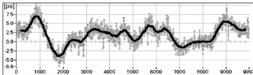
**Figure 3.** A033-ET integral non-linearity errors over interpolation interval
