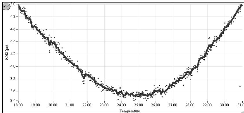
**Figure 4.** A033-ET RMS resolution vs. ambient temperature variation
