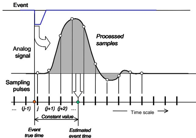
**Figure 1.** Principle of DSP-based method for event timing
