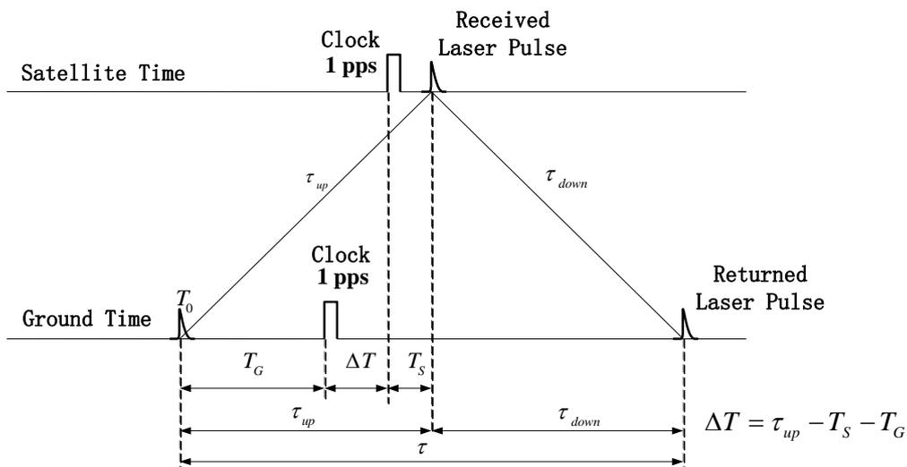
Figure 8. The principle of Laser Time Transfer, where:
