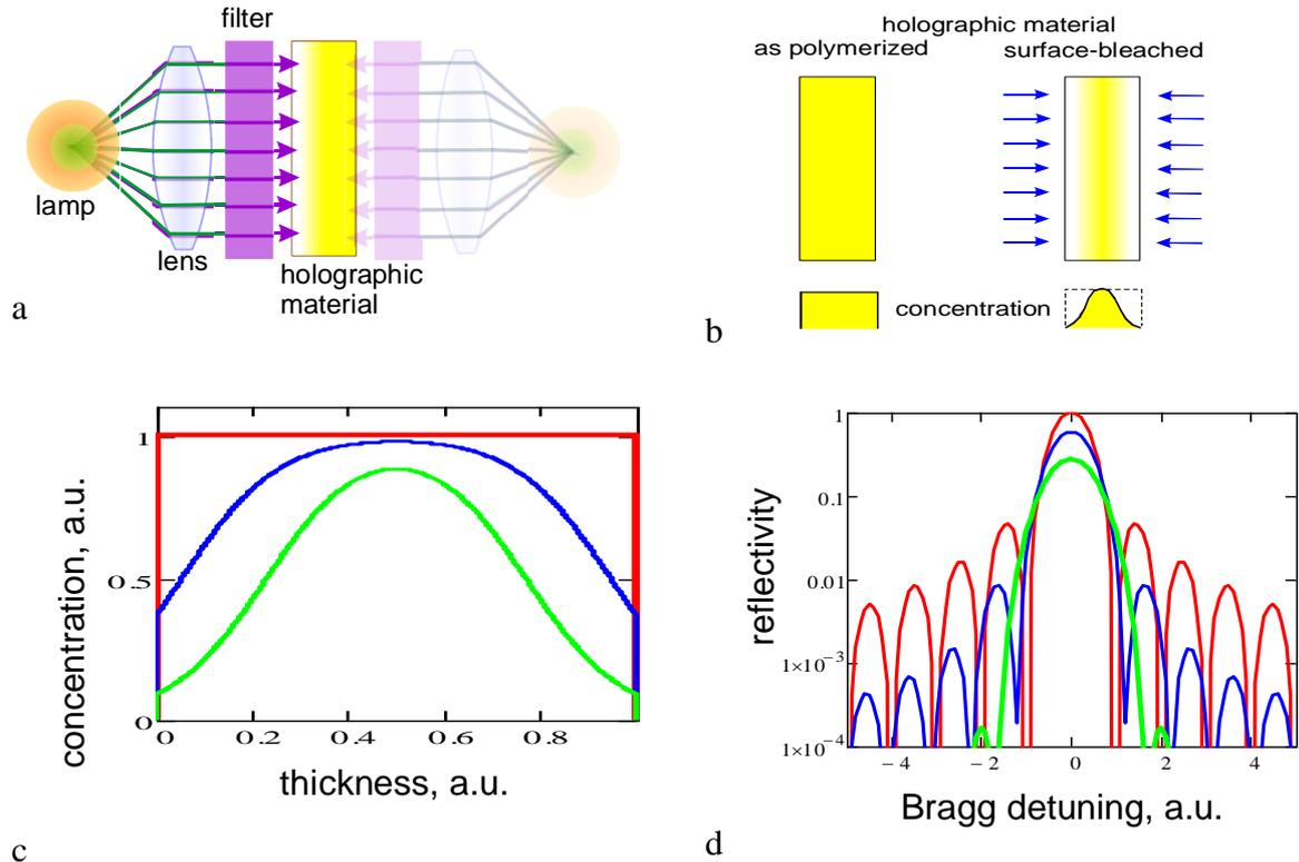
**Figure 4.** Photoapodization: schematic representation of pre-exposure treatment (a, b), light-sensitive centers distribution at different depths of apodizing treatment (c) and corresponding selective response functions of holographic gratings recorded in thus “apodized” material (d)
