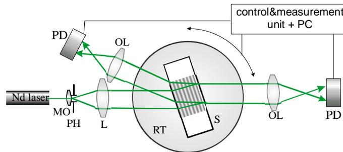
**Figure 7.** Optical arrangement of the angular selectivity measurement: Nd laser, collimator consisting of lenses, rotary table RT , objective lenses OL collecting transmitted and diffracted light on the two photodetectors PD, and the electronic unit responsible for controlling the stepping motor, signal acquisition and its transfer to the computer.
