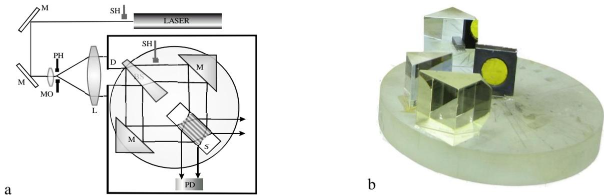
**Figure 5.** Optical layout (a) and general view (b) of the interferometer used for the hologram recording
