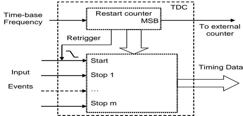
**Figure 1.** A TDC with Additional Restarting Circuitry
