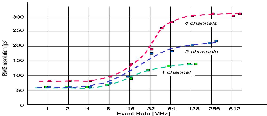
**Figure 5.** RMS Resolution vs. Aggregate Input Event Rate
