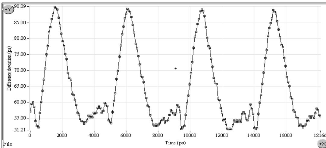
**Figure 7.** Non-linearity of Time Measurement
