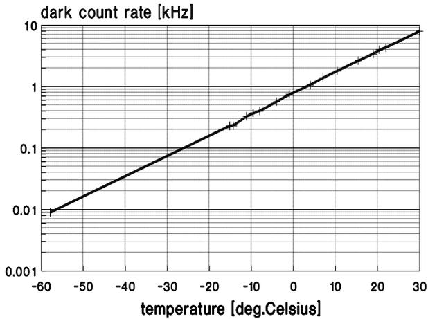
**Figure 3.** The detector dark count rate as a function of chip temperature, SPAD 25  $\mu\text{m}$  in diameter biased 0.7 V above, the slope corresponds to a drop of dark count rate of one decade per 30 K.
