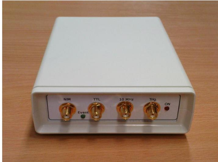
**Figure 2.** The front panel of the timing unit.
