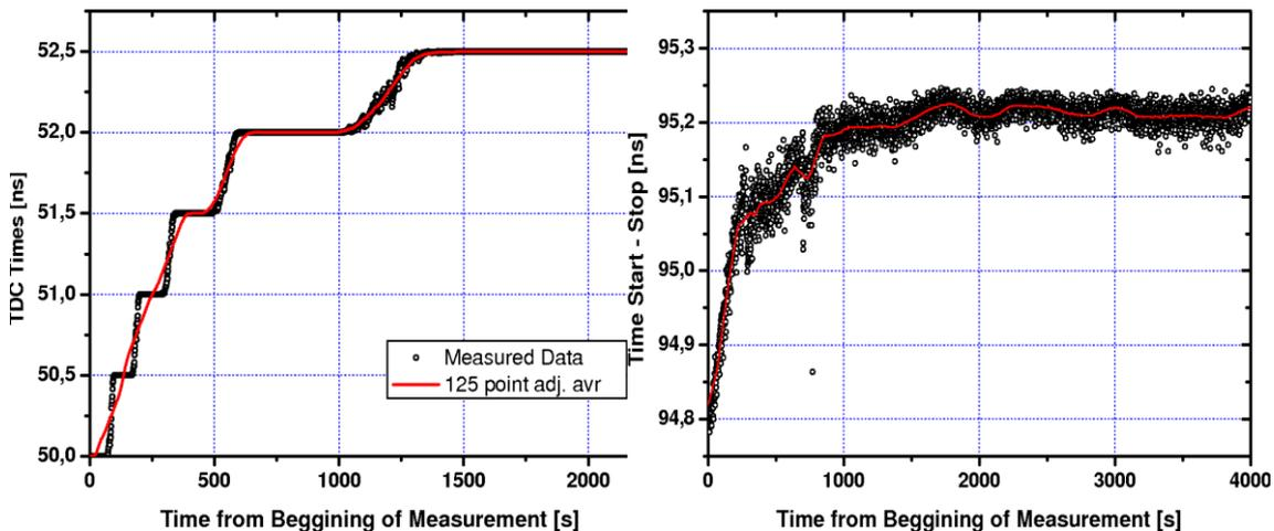
**Figure 6.** The first graph shows the warm up characteristics of the timing unit in event timing regime. Each point represents average of 255 samples. The second graph shows the warm up characteristics of timing unit in start - stop regime. Each point represents average of 255 samples.
