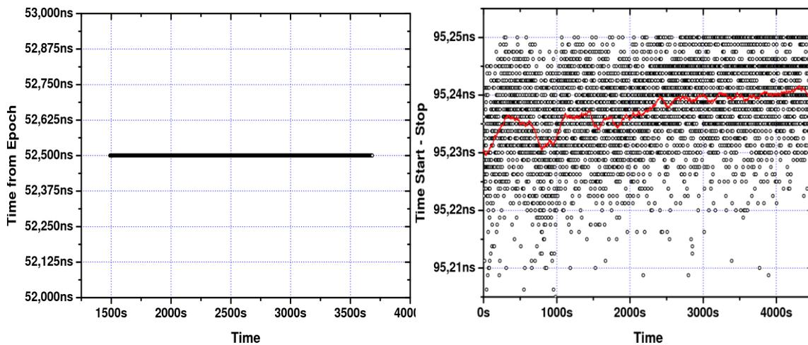
**Figure 7.** The first graph shows the long term stability of event timing. Each point represents average over 255 points. The second graph shows the long term stability of time intervals measurement. Each point represents average over 255 points and adjacent averaging over 100 points was applied.
