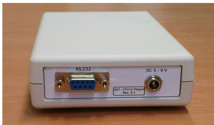
**Figure 3.** The back panel of the timing unit.
