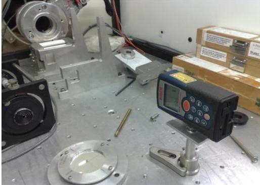
An adjustable mount was manufactured enabling the Rangefinder to be aligned to reflect correctly off all mirrors and measure directly the required coude path length.
