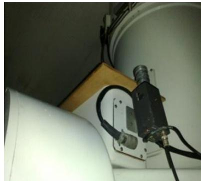
Emitter removed and replaced with flat surface.
