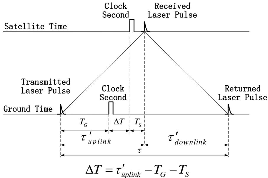
**Figure 1.** Principle of Laser Time Transfer (LTT)
