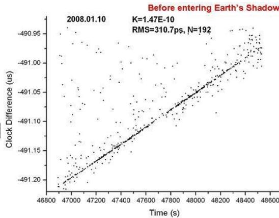
**Figure 7.** Clock differences before Earth's shadow on Jan 10, 2008
