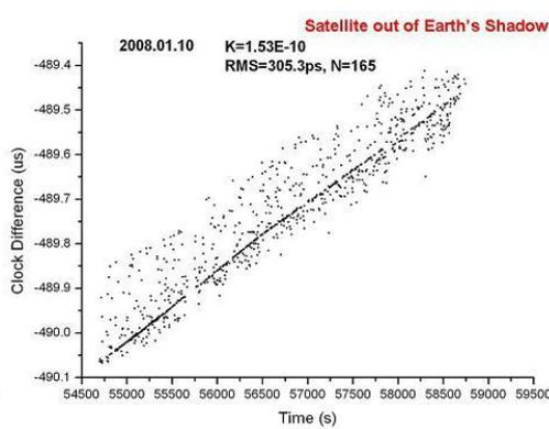
**Figure 9.** Clock differences after Earth's shadow on Jan 10, 2008
