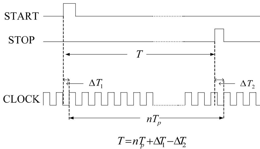
Figure 1. Interpolating Principle
