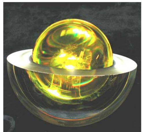
Figure 7. 17 cm-diameter spherical retrereflector (dissembled)
