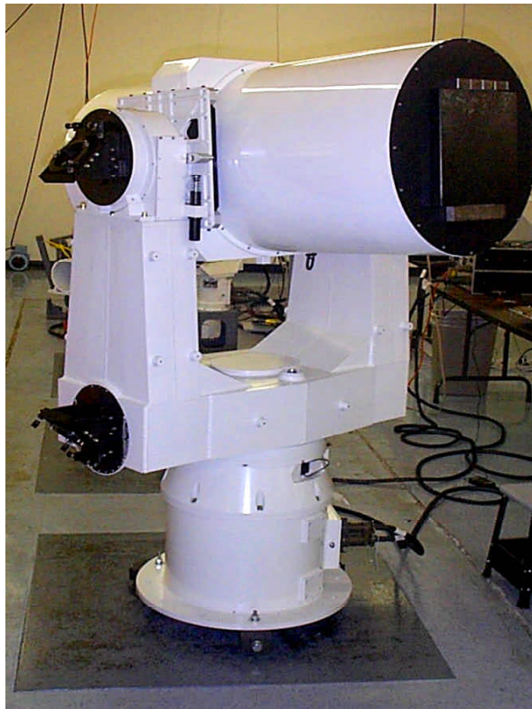
Mount with the Mass Simulator (Duplicates telescope size, weight, inertia)
