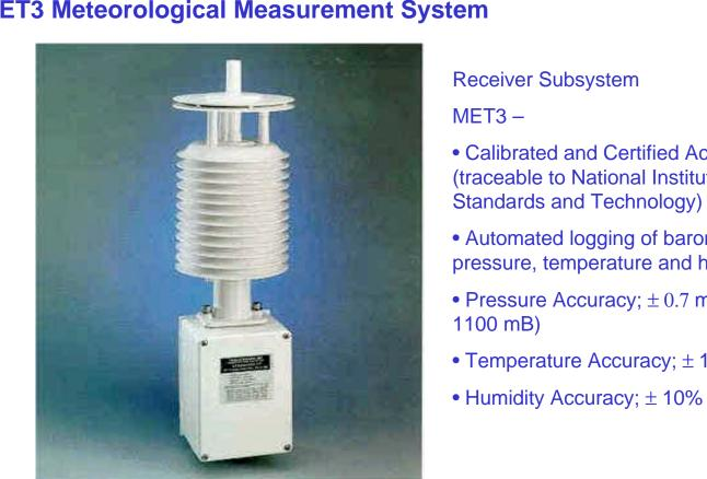
Receiver Subsystem MET3 - Calibrated and Certified Accuracy (traceable to National Institute of Standards and Technology) Automated logging of barometric pressure, temperature and humidity • Pressure Accuracy; ± 0.7 mBar (600 1100 mB) Temperature Accuracy; ± 1 degree (
