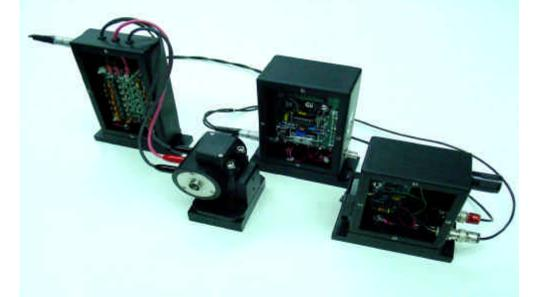
Laser Subsystem Pulse Slicer -• Eliminates Krytrons ( longer produced) • Reduces Maintenand
