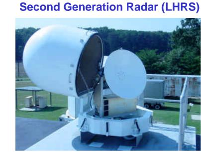
Mount Subsystem Second Generation Radar (LHRS) - Replaced FSK Modems with COTS Added Watchdog Circuitry to Microprocessor Power Supply Upgrades Laptop PC Maintenance and Operati
