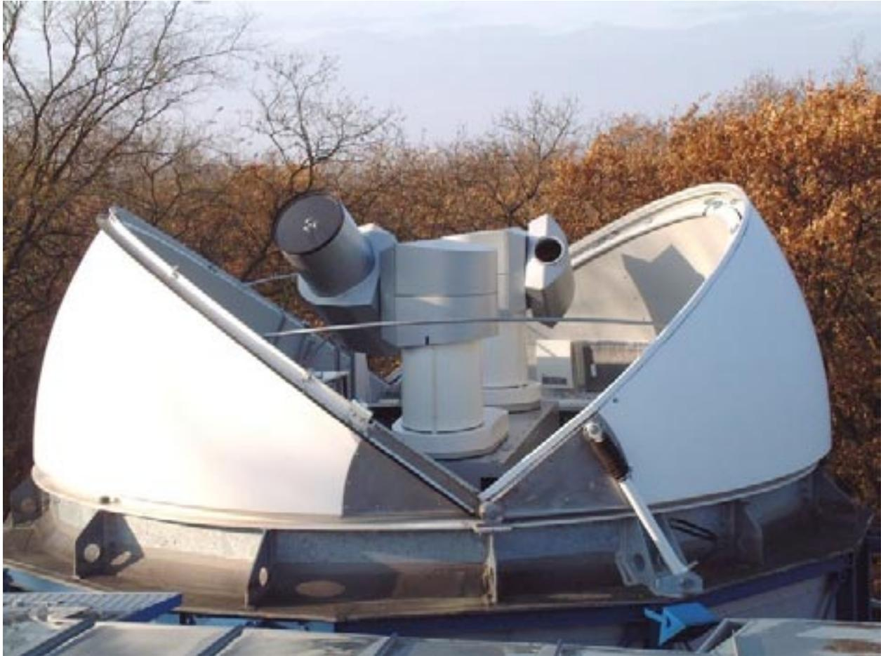
**Figure 1 Transmit and receive telescopes of the new Potsdam SLR station**
