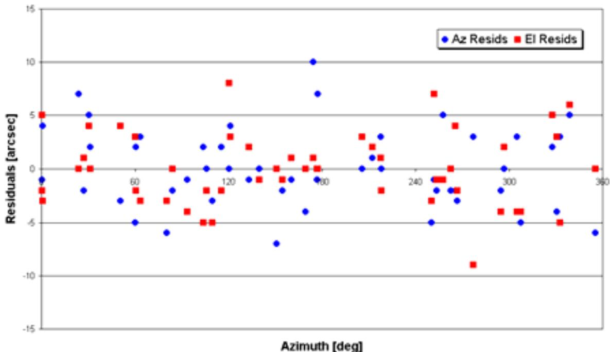
**Figure 5** Residuals in azimuth and elevation for a field of 50 stars as measured by the transmitter telescope, RMS ~3.5 arcsec for both axes (using 17 model parameters)
