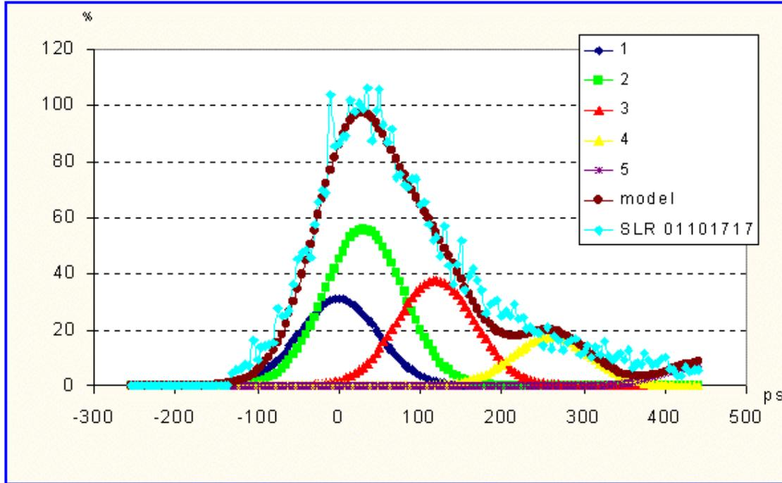
**Figure 9:** LAGEOS –2 pass (17<sup>th</sup> October 2001). Comparison between the OCA SLR raw data (cyan) and the computed model (brown). The contribution of each row up to the 5<sup>th</sup> to the satellite response are also indicated.
