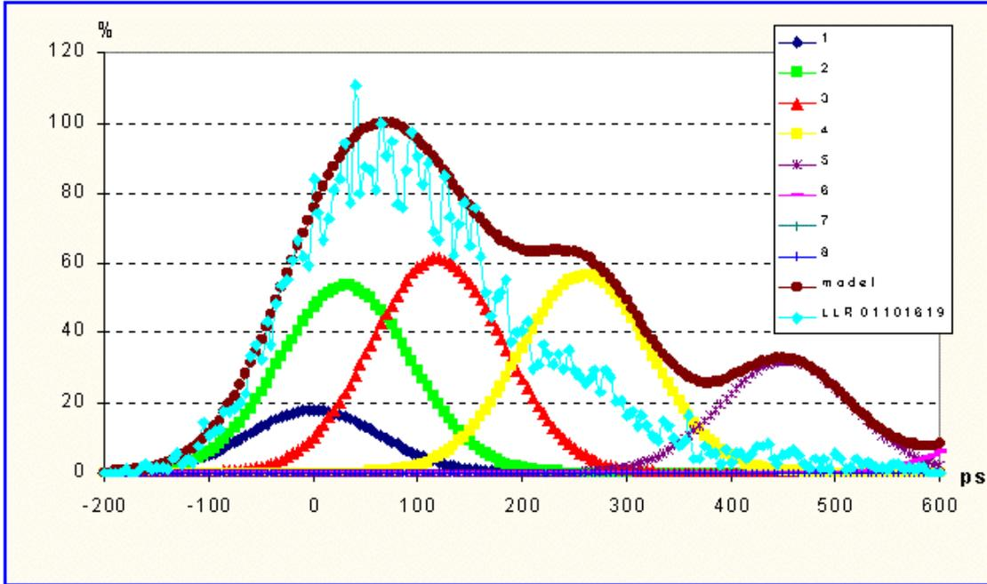
**Figure 7:** LAGEOS –2 pass of the 16<sup>th</sup> October 2001. The contribution of each row of CCRs up to the 8<sup>th</sup> and the final model obtained with the convolution of each row contribution (in brown) are represented. The cyan curve corresponds to the real raw data observed by the OCA LLR station.
