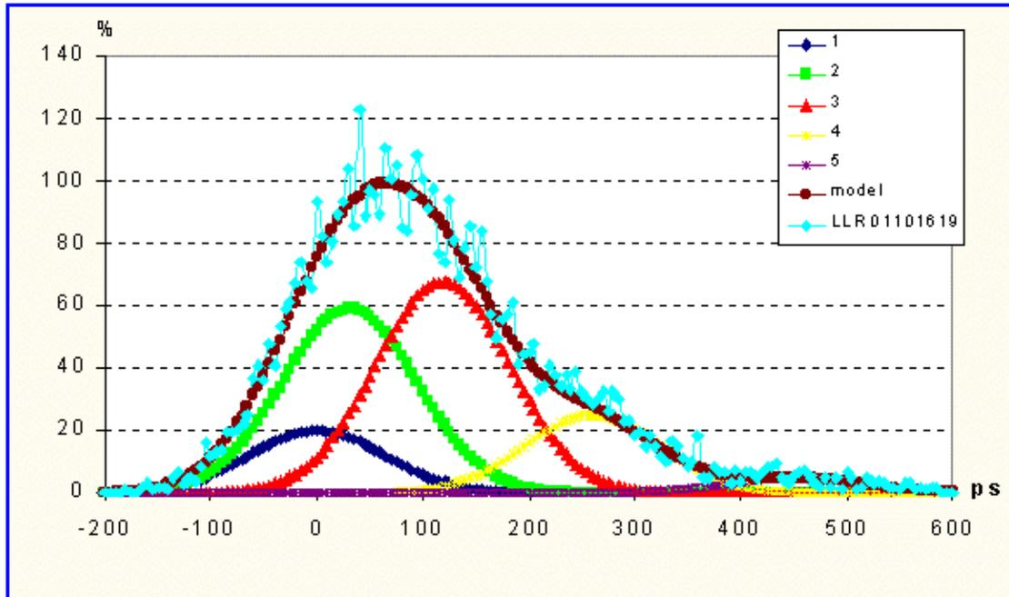
**Figure 8:** Comparison between the LAGEOS –2 LLR raw data (pass of the 16<sup>th</sup> October 2001) and the satellite response model with the attenuation factors. The contribution of each row up to the 5<sup>th</sup> are also indicated.
