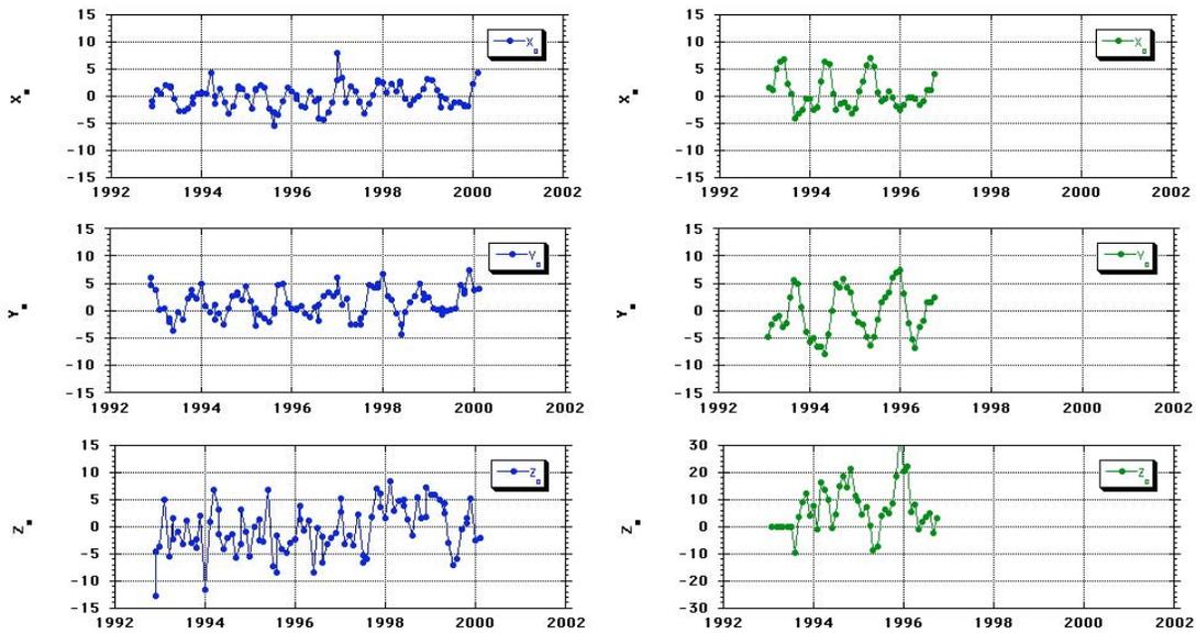
**Figure 4.** The monthly mean geocenter series from CSR/UTEX (left) based on the combined reduction of SLR and DORIS data, and from CNES (right), from DORIS data alone (note scale change for z-component of CNES).
