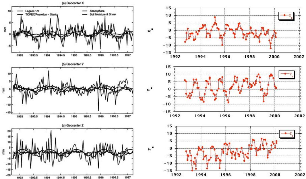
**Figure 3.** The CSR/UTEX 12-day (left) and monthly (right) series of observed geocenter components from LAGEOS-1 and -2 solutions, along with atmospheric, continental hydrological and oceanic contributions [Chen et al., 1999].
