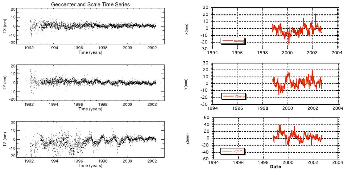
**Figure 5.** The daily mean geocenter series from JPL (left, in cm) based on the reduction of GPS data from the global IGS network, and the weekly mean estimates from the IGS Analysis Coordination Center (right, in mm) [Ferland, R., 2003].
