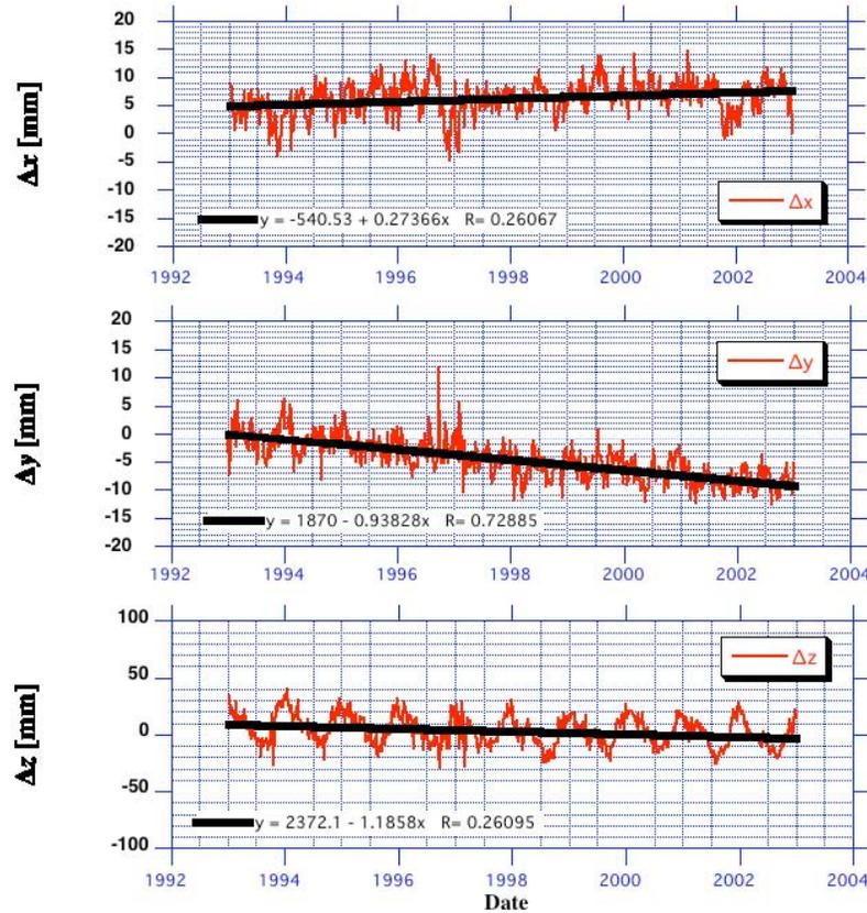
**Figure 2.** JCET/GSFC weekly average geocenter offsets based on the analysis of LAGEOS and LAGEOS-2 SLR data over 1993.0 - 2003.0 (Note: these are total variations, including trends).
