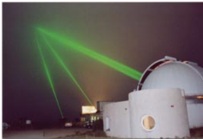
Figure 2: The 3 OCA laser ranging station during the collocation campaign simultaneously tracking the LAGEOS satellites. From the left to the right: the French Transportable Laser Ranging Station (FTLRS), the Satellite Laser Ranging (SLR) station, and the Lunar Laser Ranging (LLR) station.
