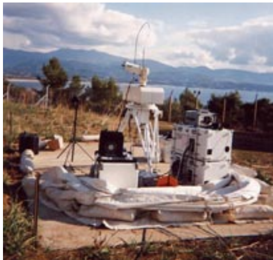
Figure 1: The French Transportable Laser Ranging Station (FTLRS).
