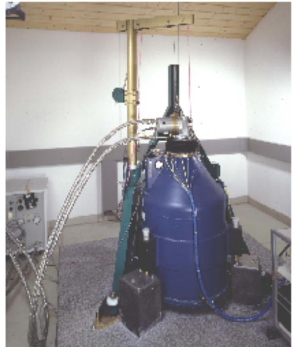
*Fig. 11: Super conducting gravity meter to measure the Earth tides during operation at Wettzell.*
