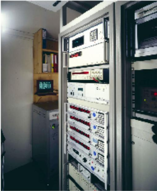
*Fig. 10: Time keeping laboratory of TIGO. In the back one of two H-masers, in the foreground one sees one of the two cesium-standards and a number of clock-modules which provide precise Universal Time.*
